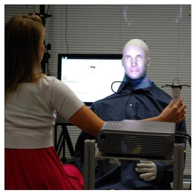
**Figure 1.** User performing an ophthalmic examination on a Shader Lamps Virtual Patient (SLVP).
