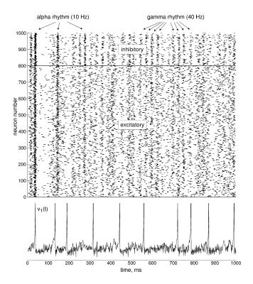
Fig. 3. Simulation of a network of 1000 randomly coupled spiking neurons. Top: spike raster shows episodes of alpha and gamma band rhythms (vertical lines). Bottom: typical spiking activity of an excitatory neuron. All spikes were equalized at  $+30 \, \mathrm{mV}$  by resetting  $v_1$  first to  $+30 \, \mathrm{mV}$  and then to c.
