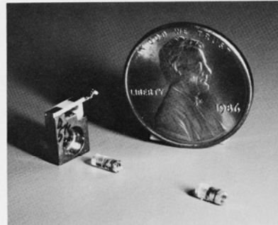
Fig. 1. (Top) Schematic of the diode laser-pumped monolithic Nd:YAG oscillator. (Bottom) Photograph of the three components that constitute the laser source: the diode laser, the gradient index lens, and the Nd:YAG crystal (5 mm long) with mirrors polished and coated on its ends.
