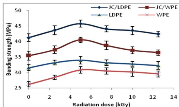
**Figure 7.** Effect of gamma radiation on the bending strength of the composites and polymer matrix sheets
