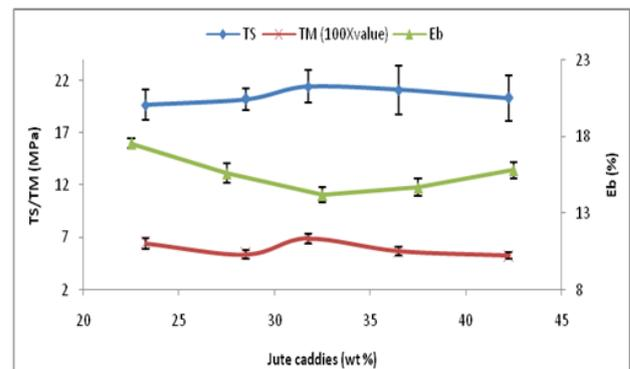
Figure 4. Effect of jute caddies content on the tensile properties of the composite (JC/WPE)
