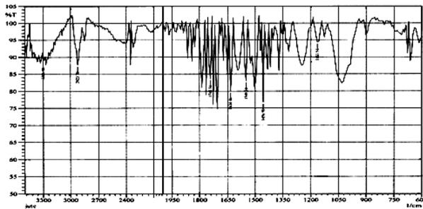
Figure 3. FT-IR spectrum of jute caddies
