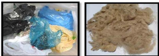
Figure 1. Waste polyethylene shopping bags and jute caddies
