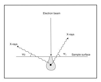
data to account for x-ray absorption and secondary fluorescence in the sample. Mass absorption coefficients are still a matter of controversy and one of the major sources of uncertainty in all correction schemes.
