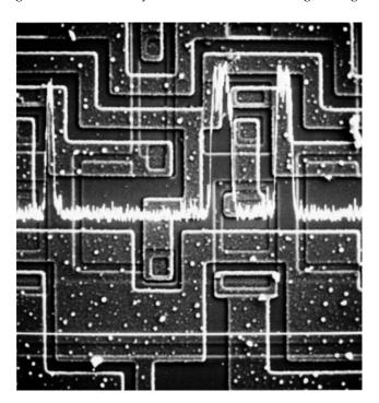
Figure 5-5. A silicon line profile for a portion of an integrated circuit. The upper trace shows the relative intensity of silicon x-rays detected as the primary beam scanned the straight line in the lower half of the photomicrograph.
