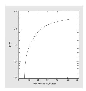
**Figure 3-3.** Plot of  $e^{-csc}\Psi$  as a function of take-off angle  $\Psi$ . As expressed in Beer's law, the probability of x-ray absorption is directly proportional to  $e^{-d}$ , where d here is proportional to  $csc}\Psi$ .
