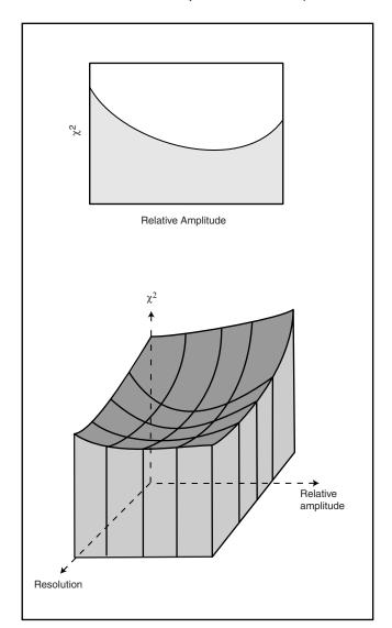
Figure 5-15. Generalized plots of  $\chi^2$  as a function of one and two variables. Minimizing  $\chi^2$  by varying only relative peak amplitude (upper drawing) is equivalent to restricting the search to a single slice of the surface in the lower drawing.
