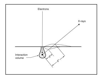
Figure 5-17. Illustration of the dependence of the absorption path length (d' and d") on sample topography. The drawing also reflects the typical computational assumption that all x-rays originate from a single point within the interaction volume.
