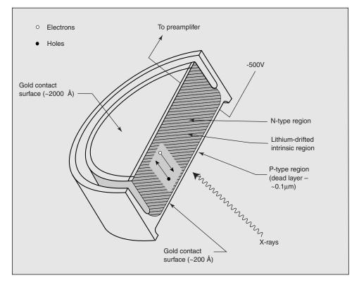
applied electric field. Therefore, whereas a pure and perfect crystal conducts very little current, an imperfect one allows some current to pass. Ideally, a crystal of perfect structure and the highest purity is used for x-ray detection.
