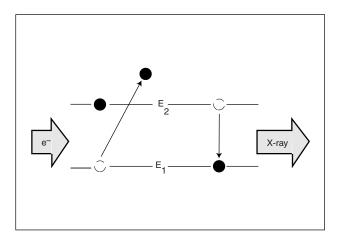
principle is a simple one: When excited by electrons of sufficient energy, every element in a sample will emit a unique and characteristic pattern of x-rays. Furthermore, under given analysis conditions, the number of x-rays emitted by each element bears a more or less direct relationship to the concentration of that element.
