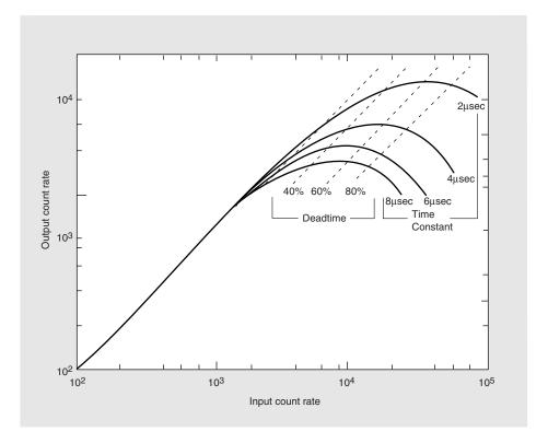
Figure 4-5. Plot of output count rate as a function of input count rate, for four pulse-shaping time constants. Because of the pulse pileup rejection circuitry, an input count rate that produces about 60% deadtime maximizes the output count rate for a given time constant.
