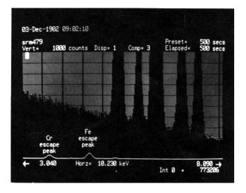
Figure 5-2. A titanium spectrum obtained at a high input count rate. Sum peaks are visible at 9.02 keV ( $K\mathbf{C} + K\mathbf{C}$ ) and 9.44 keV ( $K\mathbf{C} + K\mathbf{C}$ ). The sum peak for  $K\mathbf{C} + K\mathbf{C}$  is too small to be seen.
