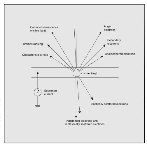
Figure 2-1. Schematic illustration of the principal results of the interaction of an electron beam with a specimen. As suggested by the figure, Auger and secondary electrons emerge from near the surface of the sample, and elastically scattered electrons are typically scattered through larger angles than are inelastically scattered electrons.
