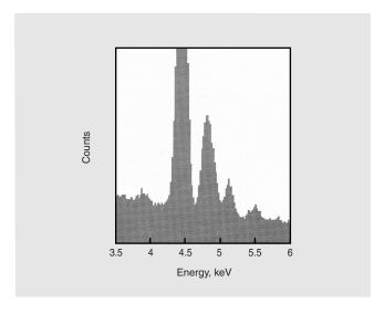
the strongest of the barium L lines are at about 4.5 and 4.8 keV. Confronted with the spectrum shown in Figure 5-3, the analyst can confirm the presence of barium on the basis of the multipeak pattern, but information about relative emission intensities is required to establish that titanium emissions contribute (or do not contribute) to the two most intense peaks. Ideally, element markers presented on the display carry this relative peak-height information.
