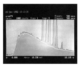
Finally, several available algorithm calculate a theoretical model of background shape, including absorption edges, then normalize the theoretical model to areas of the spectrum known not to include characteristic peak information (see Figure 5-9). This technique has proved reliable and highly accurate. It adequately accounts for most known phenomena associated with the continuum background. It has the disadvantage of being slower than other background removal techniques.
