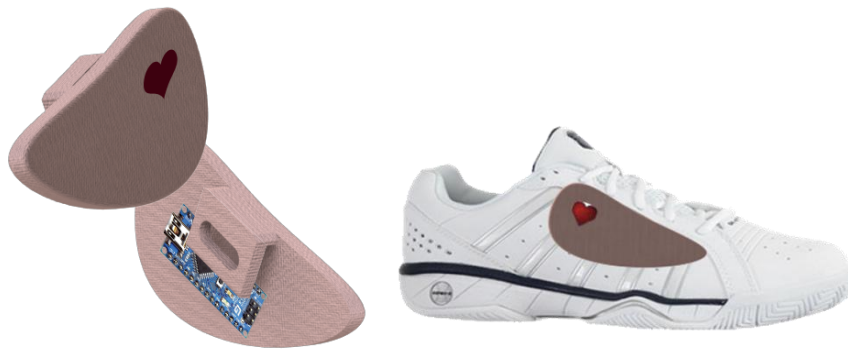
Figure 16: Mockup of accessory clip form factor
