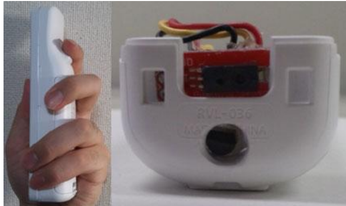
Figure 15: Latest Remote Iteration with Intended Hold and Some Sensor Placement
