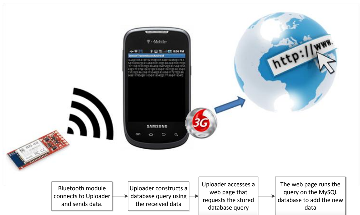
Figure 34: Flow of Data from Bluetooth to Smartphone to Internet
