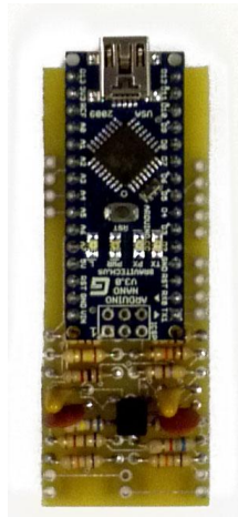
Figure 30: Printed Circuit Board Post-Installation with Arduino Nano Mounted
