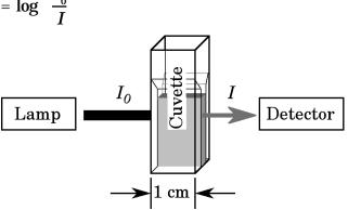
The typical internal arrangement of a Spectrophotometer
