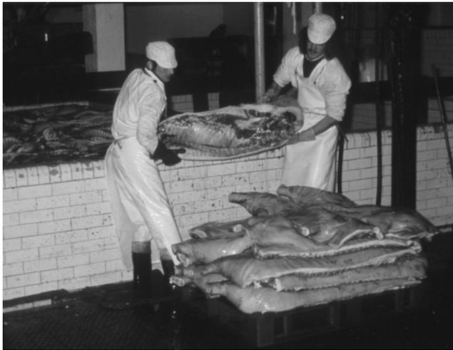
**Figure 18.1.** Traditional Wiltshire curing as practiced 50 years ago involved the manual injection of a brine into pork sides, followed by immersion in a “live brine” and maturation for about 10 days. The process was slow and labor intensive.
