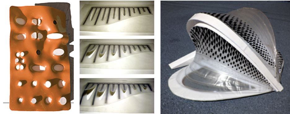
Figure 5.7, Wayne Jenski Studies (Left to Right): Silicon & HDPE; Manganese & Invar Bimetal Strips within Silicon
