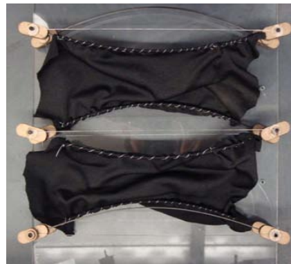
Figure 7.9, Bistable Assembly 03 Model - CFRP Strip & Rod / Polyester - Nylon Fabric / Tension Line / Composite Pin Connection
