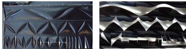
Figure 6.18, Bi-laminate Membrane With Different Coefficient of Thermal Expansion - Greg Blonder, Blonder Inventions, LLC, New Jersey
