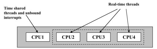
**Figure 2: Solaris Processor Binding and Control**
