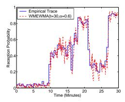
Figure 3: WMEWMA( $t = 30, \alpha = 0.6$ ) with stable setting using empirical traces.
