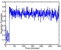
(b) After 20 minutes, the sender is moved from 15 ft to 8 ft from the receiver and remained stationary for four hours.
