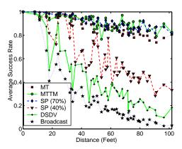
Figure 11: End-to-End success rate over distance from simulations.
