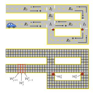
Fig. 5. The road network and its partition for the autonomous vehicle example. The solid (black) lines define the states in the set  $\mathcal V$  of the finite state model  $\mathbb D$  used by the trajectory planner. Examples of subsets  $\mathcal W_j^i$  are drawn in dotted (red) rectangles. The stars indicate the positions that need to be visited infinitely often.
