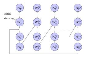
Fig. 3. A graphical description of the receding horizon strategy for a special case where for each  $i \in I_g$ ,  $\mathcal{W}^i_j \prec_{\psi_{g,i}} \mathcal{W}^i_k$ ,  $\forall j < k$ ,  $F^i(\mathcal{W}^i_j) = \mathcal{W}^i_{j-1}$ ,  $\forall j > 0$  and  $F^i(\mathcal{W}^i_0) = \mathcal{W}^i_0$ .
