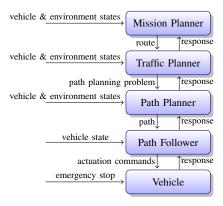
Fig. 1. A hierarchical protocol stack.
