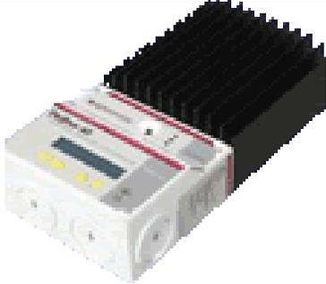
Since the brighter the sunlight, the more voltage the solar cells produce, the excessive voltage could damage the batteries. A charge controller is used to maintain the proper charging voltage on the batteries. As the input voltage from the [solar array](#) rises, the charge controller regulates the charge to the batteries preventing any over charging.
