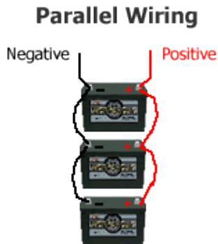
This diagram shows a simple parallel circuit to increase current or power. Assume that we are using 12 volt batteries. The power of all 3 batteries add to give us the effect of a battery 3 times as powerful but the voltage stays the same at 12 volts. Parallel wiring increases current but the voltage does not change. This is the wiring used when jump starting a car for example.
