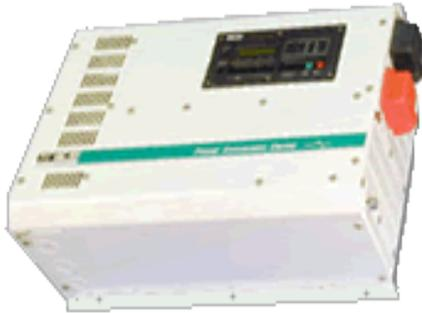
Unless you plan on using battery power directly for everything, you will need a Power Inverter. Since the majority of modern conveniences all run on 120 volts AC, the Power Inverter will be the heart of your Solar Energy System. It not only converts the low voltage DC to the 120 volts AC that runs most appliances, but also can charge the batteries if connected to the utility grid or a [AC Generator](#) as in the case of a totally independent stand-alone solar power system.
