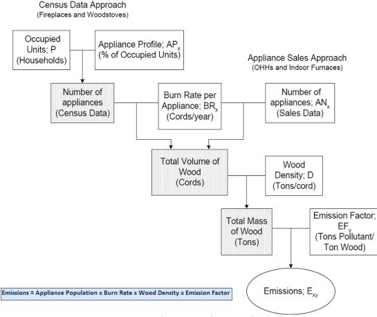
Figure 1. Data flow diagram for the RWC Tool.
