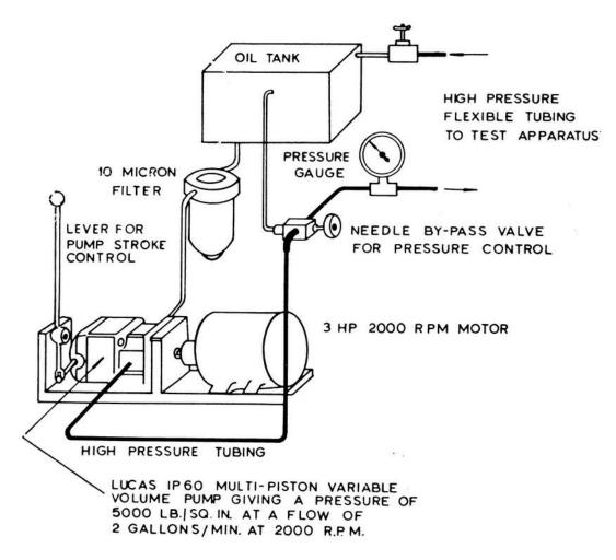
Figure 11. Circuit used for producing accurately controlled hydraulic pressures.
