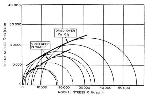
Figure 6. Mohr fracture envelopes showing the effect of moisture on the compressive strength of quarzitic shale (from Colback & Wiid)
