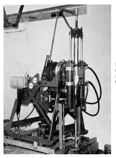
Figure 7: Drilling machine used to obtain specimens in the laboratories of the South African C.S.I.R.
