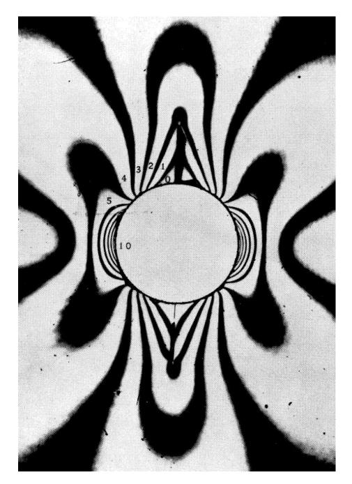
Figure 4. Photoelastic pattern in a glass plate model containing a central circular hole from which vertical tensile cracks have propagated.
