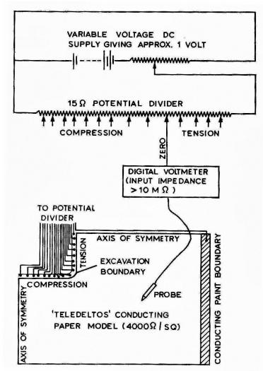
Figure 3. Circuit for conducting paper analogue.
