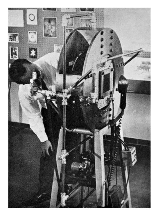
Figure14. Apparatus used by the C.S.I.R. for subjecting plate models to biaxial compressive loading.
