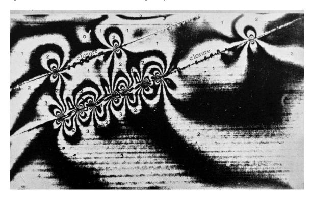
Figure 6. Photoelastic pattern in a min model which was stress-frozen at a centrifugal acceleration of 100 times the acceleration due to gravity.
