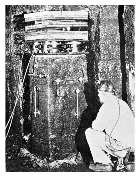
Figure 9. A large scale coal specimen under test.
