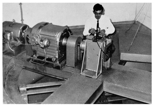
Figure 5. The C.I.S.R.'s 9 ft. diameter centrifuge for subjecting models to acceleration of up to 1,000 times the acceleration due to gravity.
