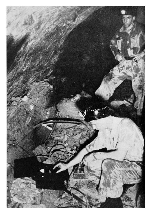
Figure 3. The measurement of stress in a deep level South African gold mine.
