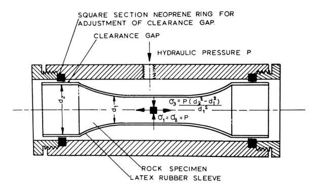
Figure 12. Apparatus for determining the tensile strength of rock specimens.
