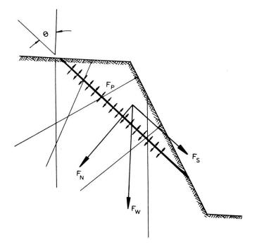
Figure 11. Forces acting on a rock slope containing a geological discontinuity
