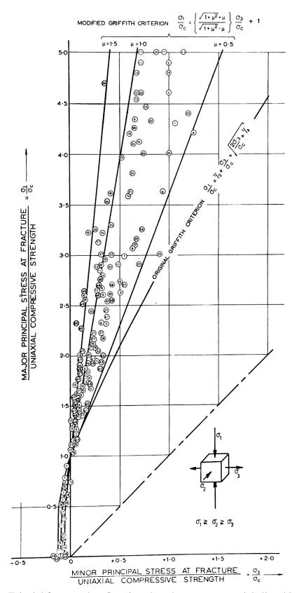
Figure 2. Triaxial fracture data for 50 rock and concrete materials listed in Table 1.
