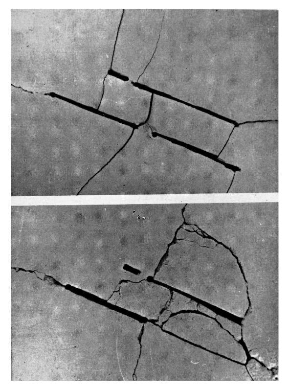
Figure 16. Comparison between the propagation of fracture in plaster of paris models subjected to uniformly distributed edge loading (upper photograph) and centrifugal acceleration (lower photograph).
