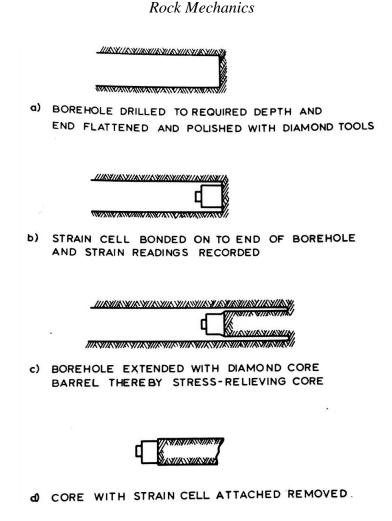
Figure 1. Sequence of operations in Leeman's method for measuring rock stress.
