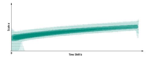
**Fig. 14.** Magnitude of the wavelet transform of a sinusoid with linearly increasing frequency.
