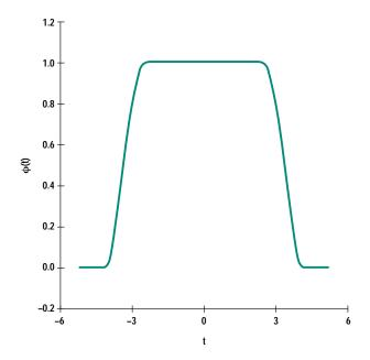
Fig. 3. Fourier transform of the scaling function for the Meyer basis.
