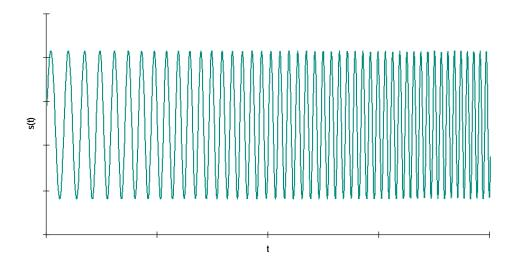
**Fig. 13.** Sinusoid with linearly increasing frequency.
