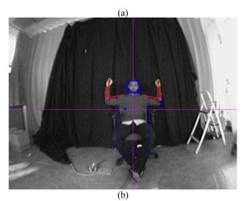
Figure 3: Example of arm pose recognition results. (a) Thresholded image detailing patchy body/arm appearance due to dark clothing. (b) Final arm angle outputs, along with face detection result.
