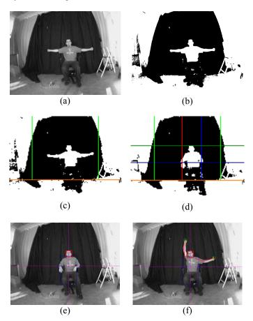
Figure 2: Steps of the arm pose recognition algorithm
