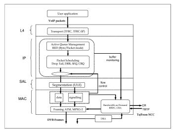
Figure 1 RCST access gateway networking diagram
