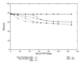
Figure 5 R-score of VoIP flows for different scheduling mechanisms.
