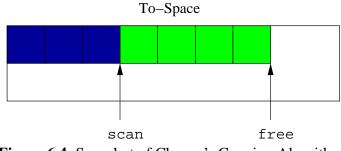
Figure 6.4. Snapshot of Cheney's Copying Algorithm
