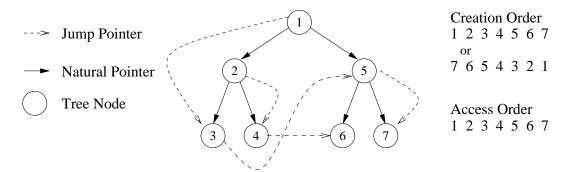
Figure 4.15. Jump-Pointer Prefetching: Binary Tree Traversal
