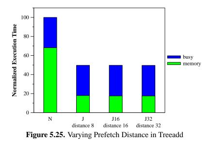
Increasing the prefetch distance from eight objects to sixteen reduces the L1 miss rate from 41% to just 2%. Unfortunately, Figure 5.25 shows that increasing the prefetching distance in treeadd from eight objects to sixteen and thirty two objects does not have an impact on execution time. The reason is that accessing the L1 cache becomes a bottleneck when we increase the prefetch distance, and many of the tree node objects are in cache when accessed.
