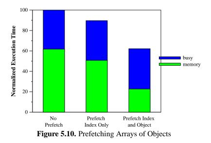
the elements and the referent objects. Prefetching just the array elements reduces execution time by just 10%. When we prefetch both the array elements and the referent objects, prefetching reduces execution time by almost 38%. This large improvement occurs even though we increase the number of instructions by issuing two prefetches and an additional load for each array reference.
