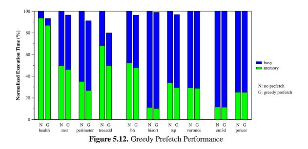
In Figure 5.12, we group the Olden programs into three sets based upon our results. We see the largest improvements in the first set of four programs, smaller improvements in the second four programs, and the final two programs do not contain significant linked structure accesses. In the programs, greedy prefetching improves performance by as much as 20% in treeadd. Across all benchmarks, we see improvements of 5% using the geometric mean.
