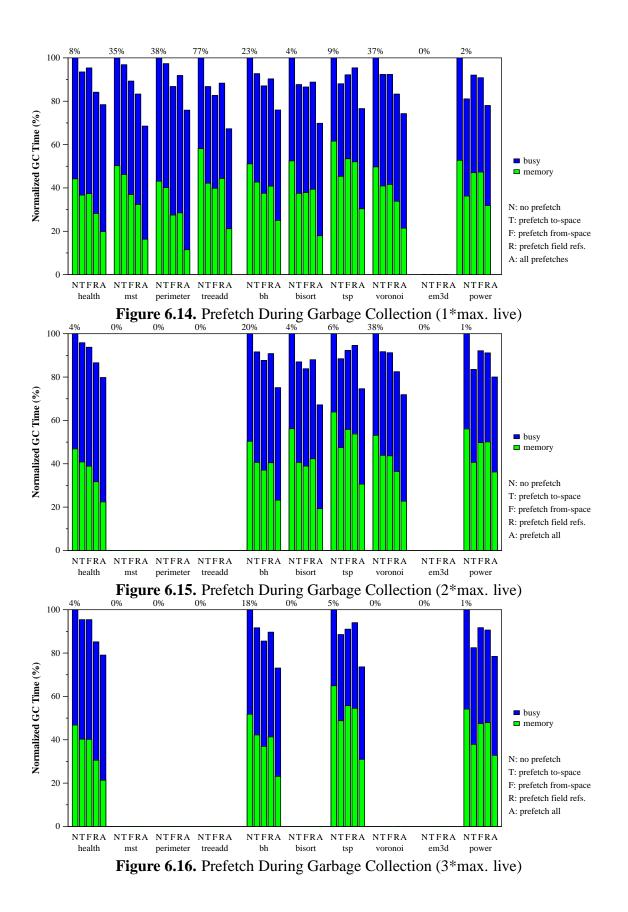
the collector. Prefetching in To-space, From-space, and in the object scan improves the collector performance by a geometric mean of 11%, 9%, and 10%, respectively. With all three prefetches, the execution time decreases by a geometric mean of 24%.
