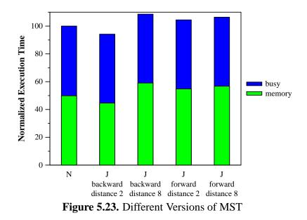
see an improvement because each linked list is small. Figure 5.23 compares the performance of mst when the compiler creates the jump-pointers in the backward and forward directions.
