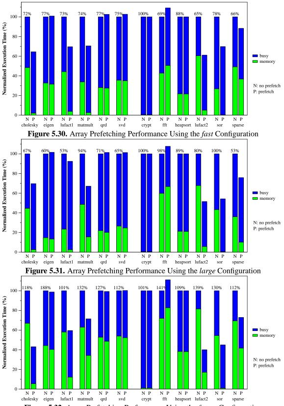
Figure 5.32. Array Prefetching Performance Using the *future* Configuration
