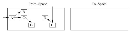
Figure 6.1. The Heap at the Start of a Collection
