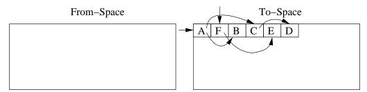
Figure 6.2. The Heap at the End of a Collection
