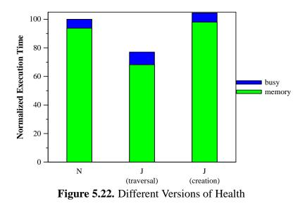
Health is the only program that both builds jump-pointers while traversing its linked structures and contains indirect recurrent variables. The jump-pointers eliminate all of the late prefetches, but we do not see larger improvements due to the overhead of updating the jump-pointers at traversal time.
