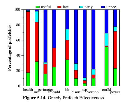
cache line is already in the L1 cache is cheap, and the additional functional units in the processor are able to hide the cost of an unnecessary prefetch.
