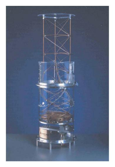
Figure 2.4: Deployment of a coilable mast from a canister by a rotating nut (Courtesy of AEC-Able Engineering Company, Inc.).
