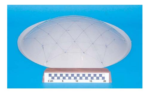
Figure 7.10: Paraboloidal plastic mold with the first of the two three-ring nets attached. The radial cables are used to connect the net to the ring structure.
