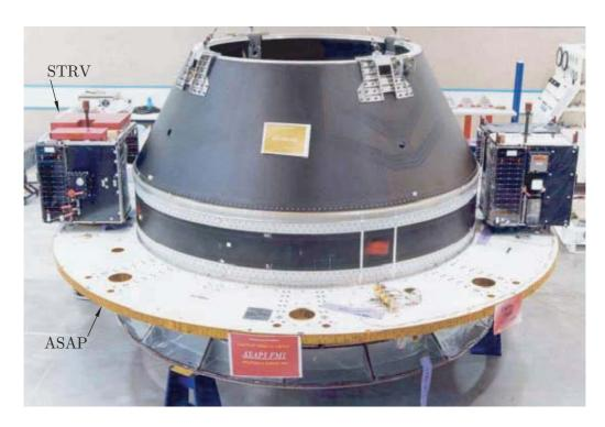
Figure 5.1: DERA's small satellites STRV-1 C and D on Ariane-5 ASAP for launcher fit check (Courtesy of DERA).
