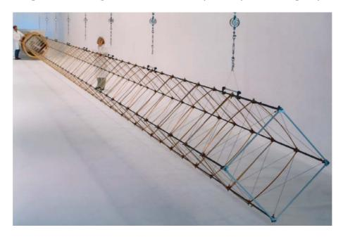
Figure 2.6: FAST mast for the ISS (Courtesy of AEC-Able Engineering Company, Inc.).
