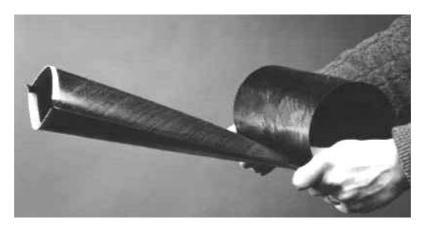
Figure 2.2: Collapsible tubular mast (Courtesy of DLR).
