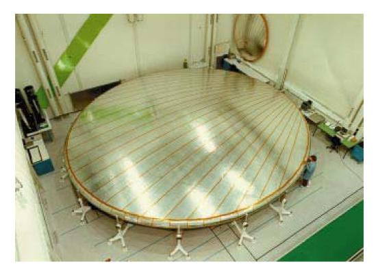
Figure 2.20: The 12 m diameter model of the inflatable space rigidised reflector antenna (Courtesy of A. G. Roederer, ESA).
