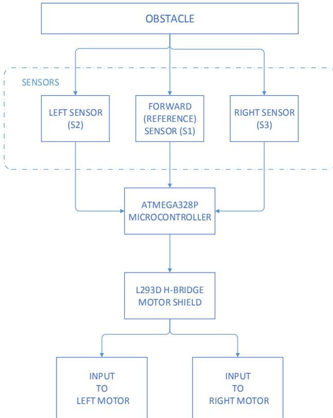
Fig. 4: Block Diagram of Obstacle Avoidance Robot
