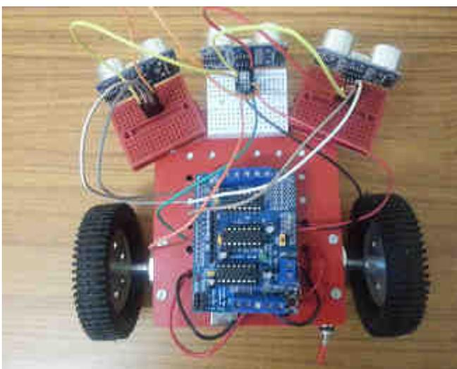
**Fig. 2: Basic Connections of the Robot.**
