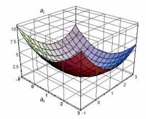
Fig. B Error surface for M=2 and filter weights  $w_1=a_0$  and  $w_2=a_1$
