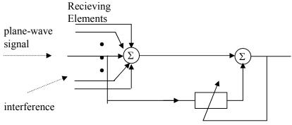
Fig. 13 ANC applied to a receiving array
