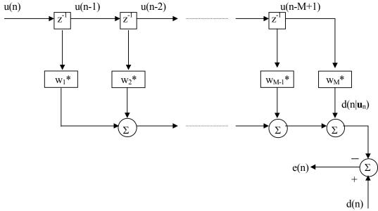
Fig.A Linear Transversal Filter
