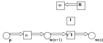
Fig. C Signal-flow graph representation of the steepest-descent algorithm.
