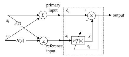
Fig. 4 ANC with signal components in reference input
