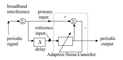
Fig. 11 ANC as self-tuning filter
