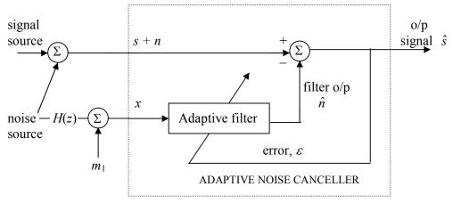
Fig. 3 ANC with uncorrelated noise in reference input
