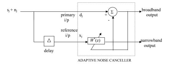
Fig. 5 ANC without reference input
