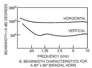
Figure 3-8. Increasing DI through narrowing vertical beamwidth
