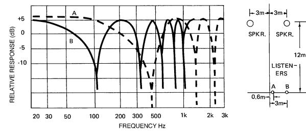
Figure 1-5. Generation of interference effects (comb filter response) by a split array
