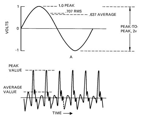
Waveform of a trumpet tone (about 400 Hz). The spread between average and peak values of the waveform is 13 dB.
