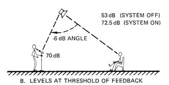
Figure 4-4. System gain calculations, directional loudspeaker
