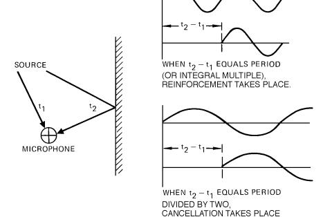
Figure 1-4A. Combining delayed signals
