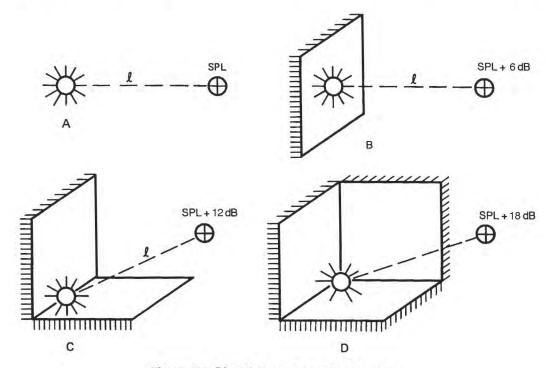
Figure 3-1. Directivity and angular coverage
