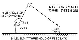
Figure 4-5. System gain calculations, directional microphone
