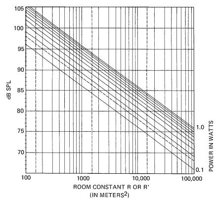
Figure 5-21. Steady-state reverberant field SPL vs.
