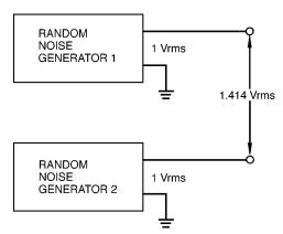
Figure 1-3. Combining two random noise generators
