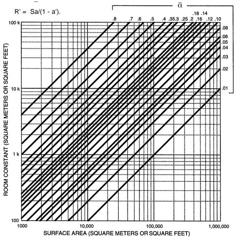
Figure 5-22. Room constant vs. surface area and
