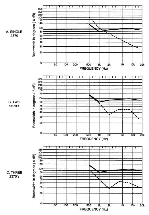
Figure 3-1 1. Stacking horns for higher directivity at low frequencies (solid line, horizontal-6 dB deamwidth, dashed line, vertical-6 dB beamwidth)
