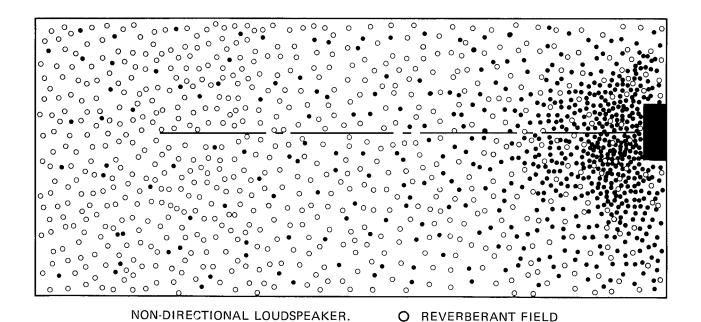
Figure 5-15. Direct and reverberant fields, non-directional loudspeaker
