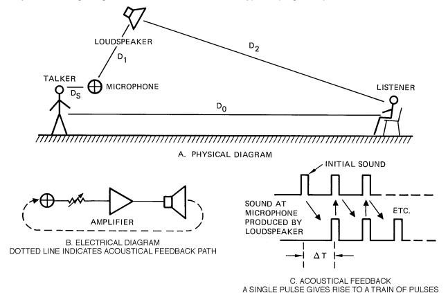
Figure 4-1. A simple outdoor reinforcement system
