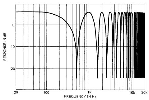
FREQUENCY RESPONSE OF TWO WIDE-RANGE PROGRAM CHANNELS COMBINED WITH ONE MILLISECOND DELAY BETWEEN CHANNELS. SAME PROGRAM SIGNAL FED TO BOTH, EXCEPT THAT AMPLITUDES DIFFER BY 0.5 dB.
