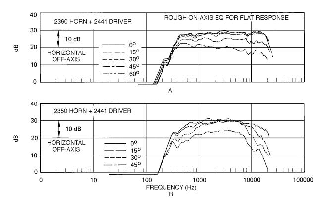
Figure 3-5. Families of off-axis frequency response curves
