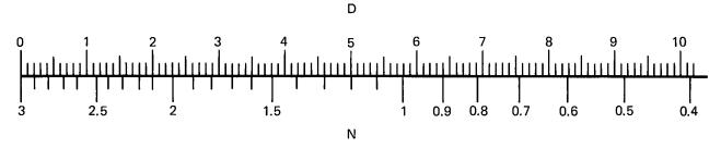
Figure 2-7. Nomograph for adding levels expressed in dB.
