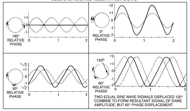
Figure 1-2. V ector addition of two sine waves
