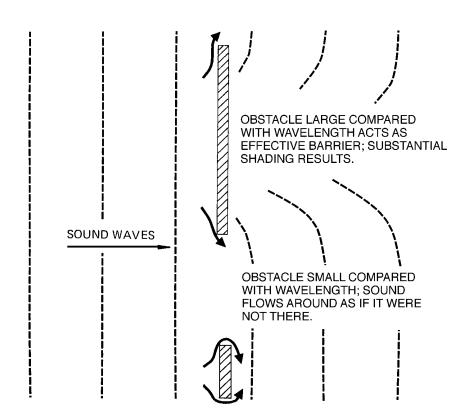
Figure 1-7. Diffraction of sound around obstacles
