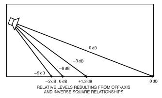
Figure 3-9. Off-axis and inverse square calculations
