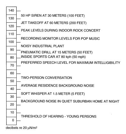
Figure 2-4.T ypical A-weighted sound levels
