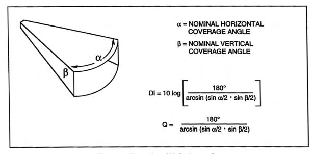
Figure 3-3. Illustration of Molloy's equation
