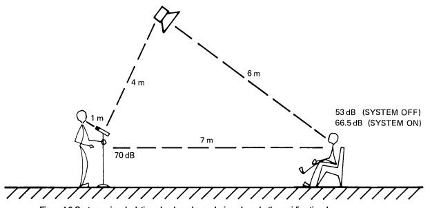
Figure 4-3. System gain calculations, loudspeaker and microphone both omnidirectional
