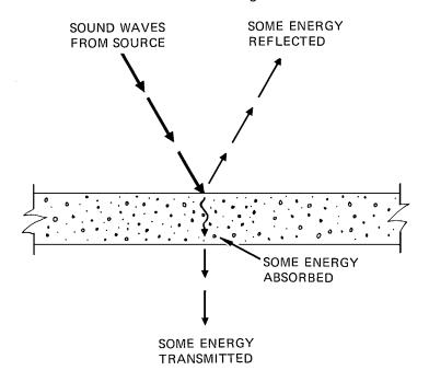
ALL THREE EFFECTS MAY VARY WITH FREQUENCY AND ANGLE OF INCIDENCE. THEY DO  $\underline{\text{NOT}}$  VARY WITH INTENSITY IN TYPICAL SITUATIONS.
