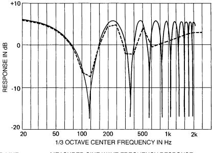
**SOLID LINE** MEASURED SINE WAVE FREQUENCY RESPONSE.
