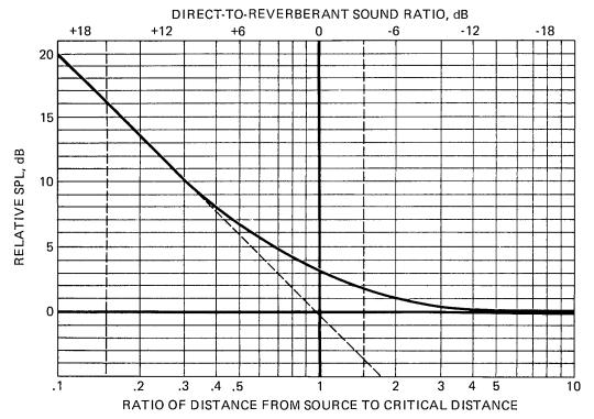
CALCULATED FROM: 10log(1+1/x<sup>2</sup>) WHERE x IS RATIO OF DISTANCE FROM SOURCE TO CRITICAL DISTANCE
