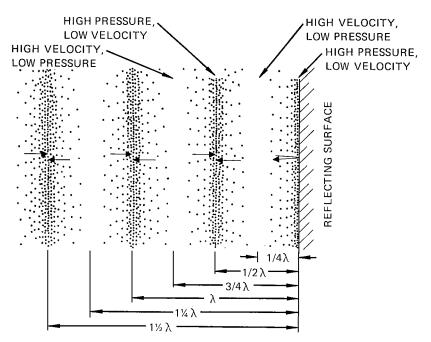
A PLANE WAVE REFLECTED FROM A PLANE SURFACE AT NORMAL INCIDENCE PRODUCES WELL DEFINED ZONES OF HIGH PRESSURE ALTERNATING WITH ZONES OF HIGH PARTICLE VELOCITY AT DISTANCES OF ONE-QUARTER WAVELENGTH
