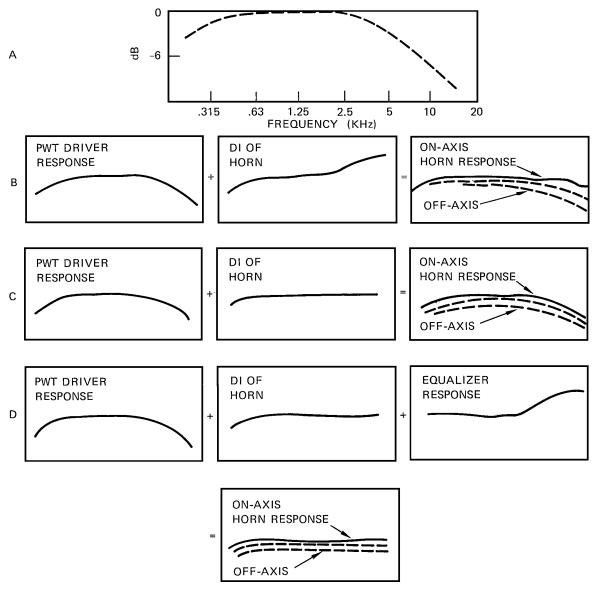
Figure 3-7. Power response of HF systems
