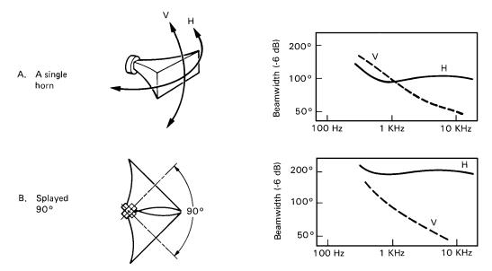
Figure 3-10. Horn splaying for wider coverage
