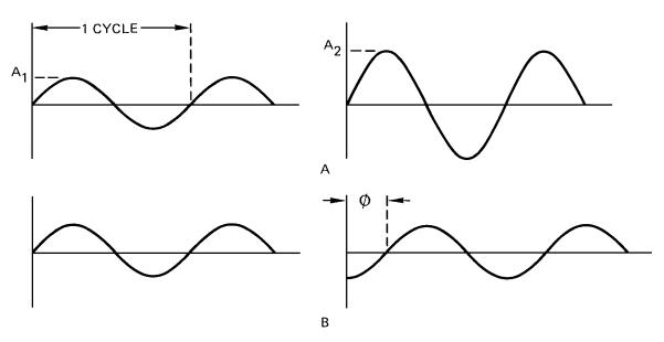
A - TWO SINE WAVES DIFFERING IN AMPLITUDE
