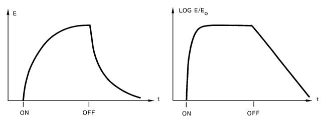
Figure 5-6. Idealized growth and decay of sound energy in an enclosure
