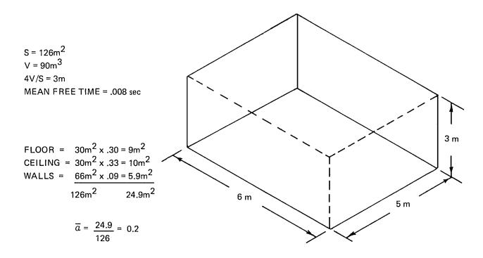
Figure 5-8. Calculating reverberation time
