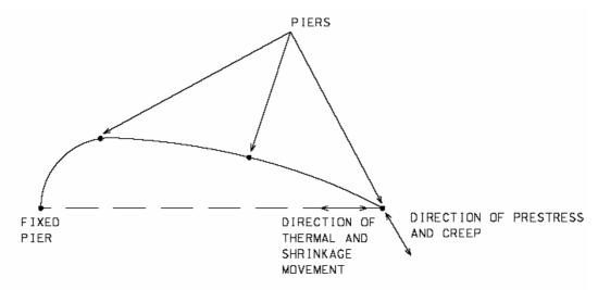
Fig. 1.2 The diagram showing how the guided bearings in piers of the curved region is oriented with respect to the fixed bearing in abutment.
