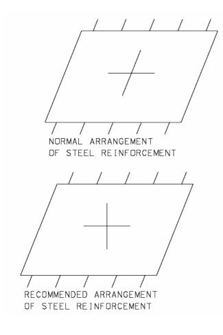
Fig. 1.3 The arrangement of reinforcement in skewed bridge.
