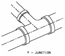
Fig. 3.4 Y-junction in drainage pipes.
