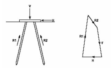
FORCE POLYGON OF A PILE BENT
