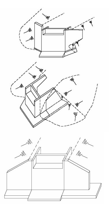
Fig. 1.4 Different orientation of wing walls.
