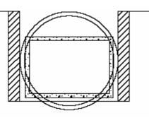
**Fig. 3.1** Small spatial requirement of box culver than pipes.
