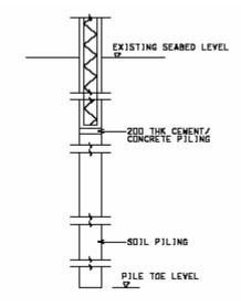
Fig. 5.1 Typical details of marine piles.
