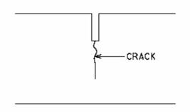
CRACK FORMATION IN UNREINFORCED PAVEMENT
