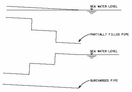
Fig. 3.2 Match soffit VS match invert.
