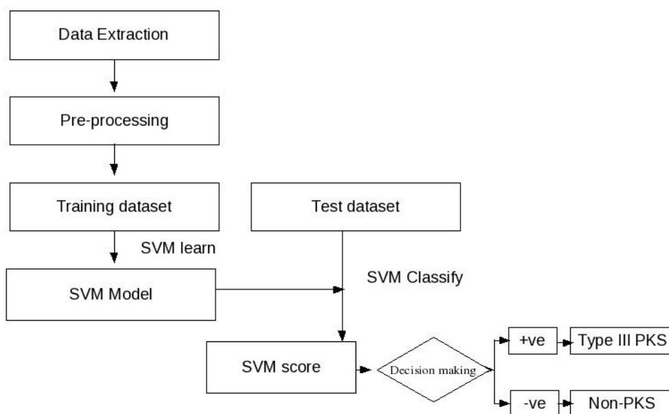
**Figure 2: The Architecture of the PKSIIIpred server.**
