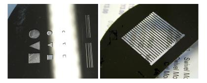
Figure 2: 2 Test structures for DRIE thru etches and trenches
