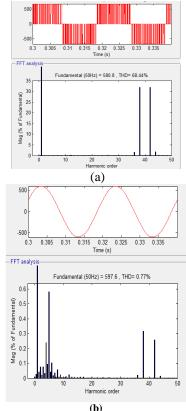
Fig. 4 Harmonics Spectrum of the Voltage Wave at 50 Hz (a) Before Filter (b) Active Filter
