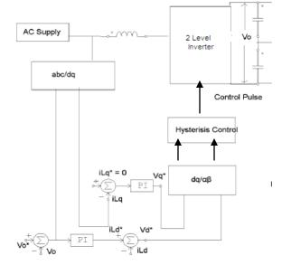
Fig.1 Control Block Diagram of AC-DC Converter
