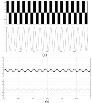
Fig. 3 Simulation Result Of Two Level AC-DC-AC Converter with IM Load (a) Line Voltage (b) Line Current at 50 Hz
