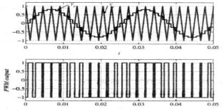
Fig. 2 SPWM: Bipolar Modulation for Two Level Inverter
