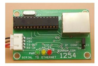
Figure 2.3. Serial to Ethernet convertor module used in the system.
