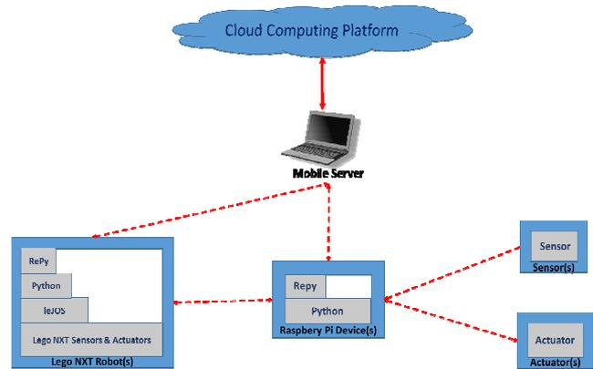
**Figure 1: Hybrid Lego NXT Mobile Cloud Robotics Architecture**
