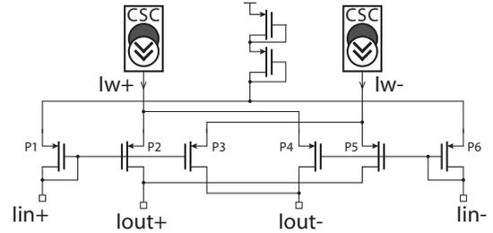
Fig. 4. Schematic of the synapse circuit (P1 = ... = P6 =  $4 \times 2$   $\mu\text{m}^2$ ).
