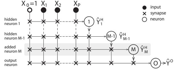
Fig. 1. The ontogenic neural network topology. The hidden neurons receive connections from both the network inputs  $X_i$  and the outputs of the previous hidden neurons  $\hat{Y}_j^H$ . The bottom neuron serves as a network output  $\hat{Y}^O$ .
