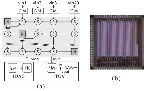
Fig. 2. (a) System architecture of the ontogenic neural network chip. The reconfigurable array of synapses (S) and neurons (N) is shown in the shaded box. (b) Die photograph of ONN chip measuring  $3 \times 3$  mm<sup>2</sup>.
