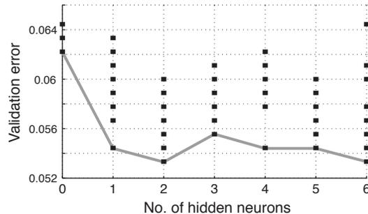
Fig. 9. The results of 10 runs of the training algorithm on the LNA task. The best validation error achieved for each number of hidden neurons is highlighted by the solid line.
