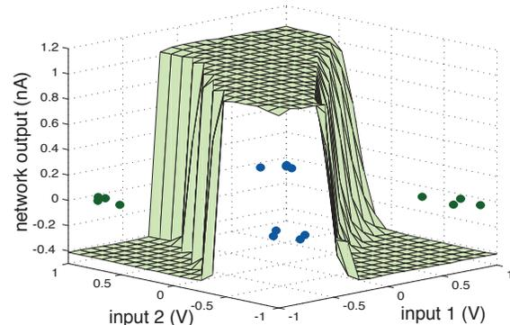
Fig. 7. Decision surface for XOR2 task obtained by measuring network output on a fine grid in input space. Also shown are the input patterns with added noise.
