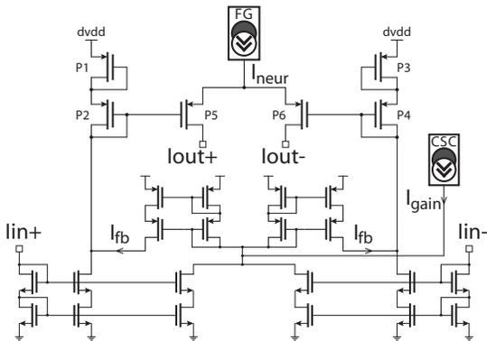
Fig. 5. Schematic of the neuron circuit. All PMOS and NMOS transistors have size  $4 \times 1 \mu\text{m}^2$ .
