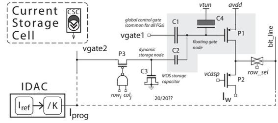
Fig. 3. Schematic of the current storage cell along with the dynamic programming loop. The sizes of key components are as follows: P1 =  $2 \times 2$   $\mu\text{m}^2$ , P2 =  $2 \times 1$   $\mu\text{m}^2$ , P3 =  $0.4 \times 0.35$   $\mu\text{m}^2$ ; C1 = 40 fF, C2 = 15 fF, C3 = 1.35 pF, C4 = 0.6 fF.
