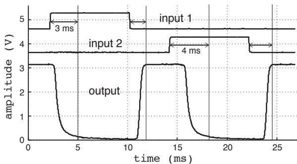
Fig. 8. Transient characteristic of the ONN trained to classify XOR2 patterns. The output is recorded from the voltage output pin of the ITOV converter.
