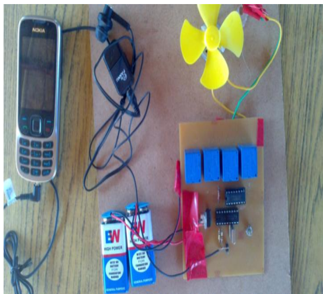
Fig.7: Hardware design for remote speed control of a DC motor by mobile
