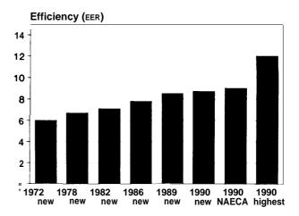
NOTES: 'New' is shipment-weighted average of all units shipped in that year. 'NAECA' is the minimum allowable according to the national standard. 'Highest' is the most efficient commercially available. See app. 2-A for a definition of EER.
