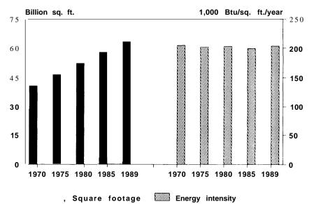
Figure I-I O-The Stock of Commercial Buildings (as measured by total square footage) Has Grown Rapidly, But the Energy Intensity (energy use per square foot per year) Has Held Steady.
