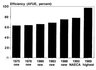
NOTES: 'New' is shipment-weighted average of all units shipped in that year. 'NAECA' is the minimum allowable according to the national standard. 'Highest' is the most efficient commercially available. See app. 2-A for a definition of AFUE.
