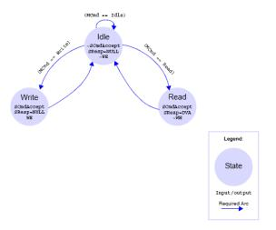
Figure 2.3. State Machine of OCP Slave
