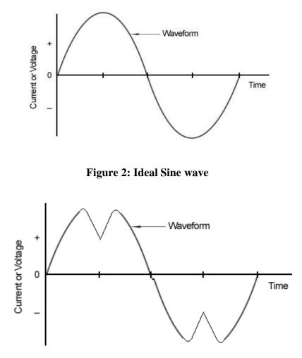
**Figure 3: Distorted Waveform**
