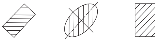
Fig. 2.11 Preferred hatching angles
