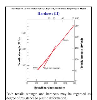
Hardness is proportional to the tensile strength - but note that the proportionality constant is different for
