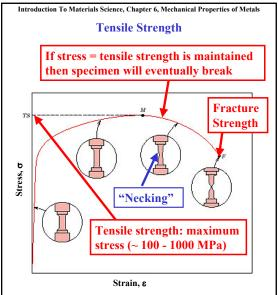
For structural applications, the yield stress is usually a more important property than the tensile strength, since once the it is passed, the structure has deformed beyond acceptable limits.
