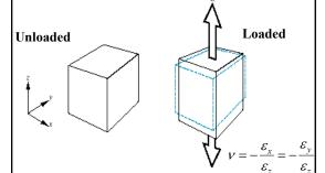
Materials subject to tension shrink laterally. Those subject to compression, bulge. The ratio of lateral and axial strains is called the Poisson's ratio  $\upsilon$ .
