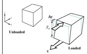
Relationship of shear stress to shear strain:
