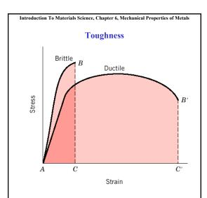
**Toughness** = the ability to absorb energy up to fracture = the total area under the strain-stress curve up to fracture
