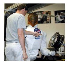
Figure 9: Execution of the pointing and labeling component of the Robonaut nut-tightening task. The four nuts are indicated by the human in order to label them with their sequence numbers, and the gestures then matched to the correct object referents simultaneously.
