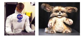
Figure 1: Humanoid robot platforms for which this deictic reference system was designed. Left: Robonaut, designed for autonomous teamwork with human astronauts in space. Right: Leonardo, designed for research into human-robot interaction.
