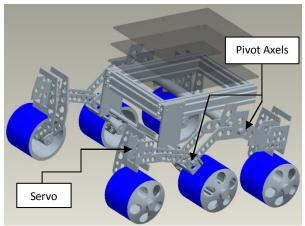
Figure-1: MIL Rover ProE model
