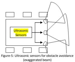
SRF04 communicates with the uC through its Trigger and Echo pins. To detect an obstacle, uC first puts a short pulse (~10ns) on SRF04's Trigger pin to tell it to ping, and then uC reads data on SRF04's Echo pin. The length of time the Echo pin stays high (5V) is used to determine whether there is any obstacle in front of the sensor.
