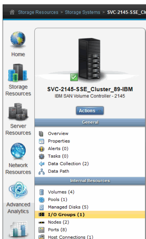
Figure 13-29 Accessing the I/O Groups view for a storage system
