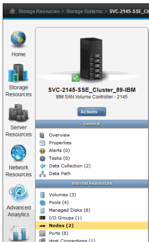
Figure 13-52 Accessing the Nodes view for a storage system
