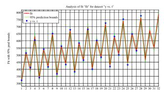
Figure 5. The plot of the stated time series together with the estimated trend (11) and 95 % prediction interval
