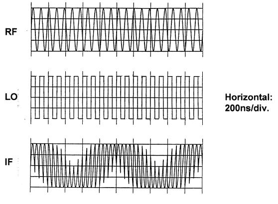
**Figure 4.5:** Inputs and Output for an Ideal Switching Mixer for  $f_{RF} = 11MHz$ ,  $f_{LO} = 10MHz$
