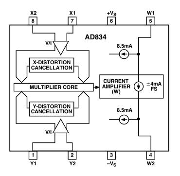
Figure 4.17: AD834 500 MHz 4 Quadrant Multiplier
