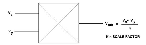
Figure 4.10: An Analog Multiplier Block Diagram
