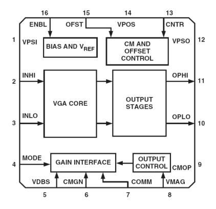
Figure 4.33: AD8330 Block Diagram
