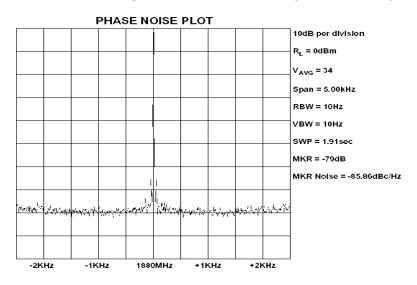
Figure 4.67: Typical Spectrum-Analyzer Output.
