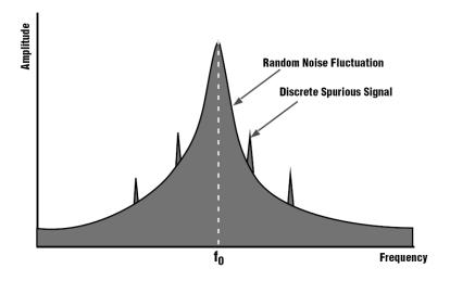
Figure 4.60: Short-Term Stability in Oscillators
