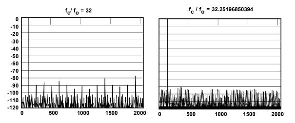
*Figure 4.46:* Effect of Ratio of Clock to Output Frequency on Theoretical 12-Bit DAC SFDR Using 4096-Point FFT
