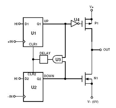
Figure 4.53: Typical PFD using D-type flip flops
