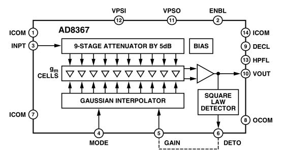
Figure 4.37: AD8367 Block Diagram
