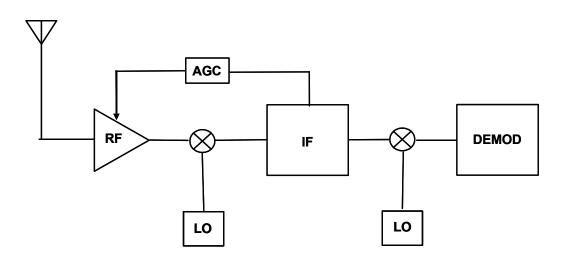
Figure 4.1: Basic Superheterodyne Radio Receiver
