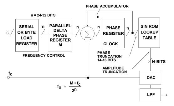
Figure 4.40: A Flexible DDS System
