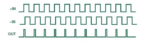
Figure 4.55: PFD waveforms, in frequency lock but out of phase lock.
