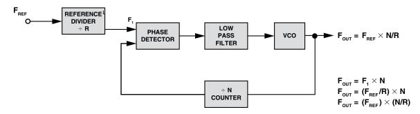
Figure 4.56: Using a reference counter in a PLL synthesizer.
