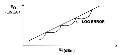
Figure 4.24: Successive Detection Log Linearity
