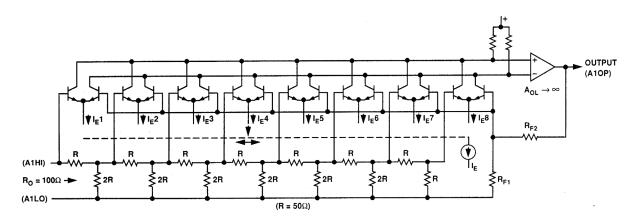
Figure 4.36: X-AMP Schematic
