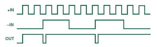
Figure 4.54: PFD waveforms, out of frequency and phase lock.
