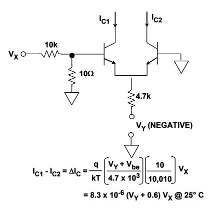
Figure 4.14: Basic Transconductance Multiplier
