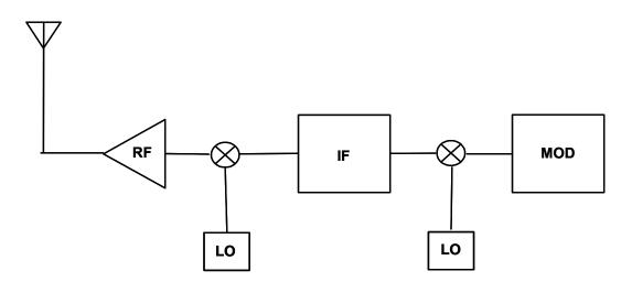
Figure 4.2: Basic Superheterodyne Radio Transmitter
