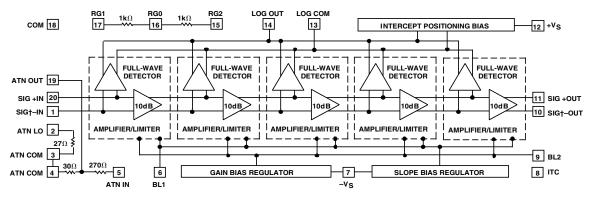
Figure 4.25: Block Diagram of the AD641 Monolithic Log Amp
