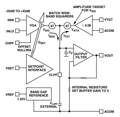
Figure 4.30: AD8362 Internal Structure
