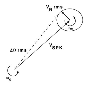
Figure 4.61: Phasor Representation of Phase Noise
