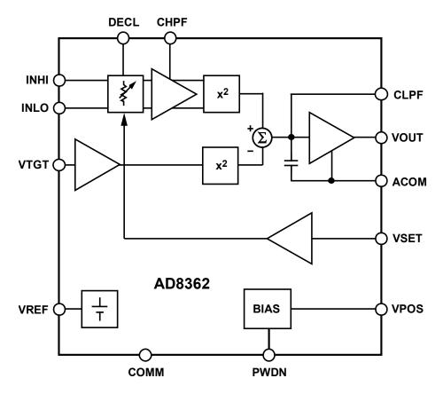
Figure 4.29: AD8362 Block Diagram
