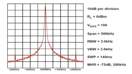
Figure 4.70: Output Spectrum Showing Reference Spurs.
