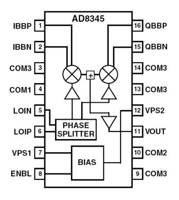
Figure 4.9: AD8345 Block Diagram
