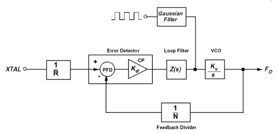
Figure 4.70: Block Diagram of Open-Loop Modulation.
