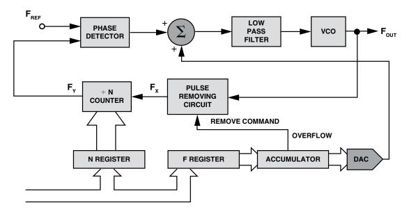
Figure 4.59: Fractional-N Synthesizer
