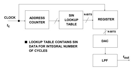
Figure 4.39: Fundamental Direct Digital Synthesis System
