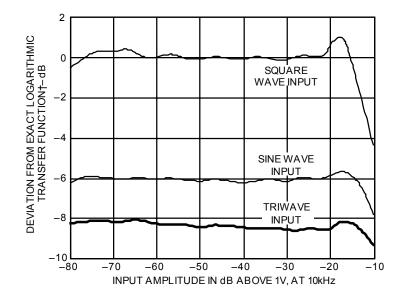
Figure 4.28: The Effect of the Waveform on AD641 Log Linearity
