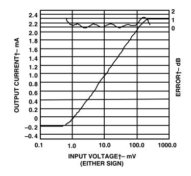
*Figure 4.26:* DC Logarithmic Transfer Function and Error Curve for a Single AD641
