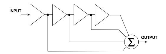
Figure 4.20: Basic Multistage Log Amp Architecture
