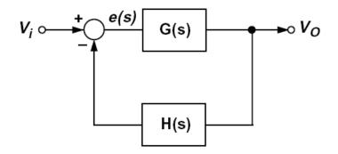
Figure 4.48. Standard Negative-Feedback Control System Model
