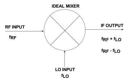
Figure 4.3: The Mixing Process
