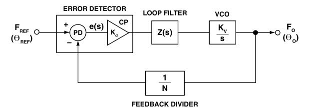
Figure 4.49: Basic Phase-Locked Loop Model.
