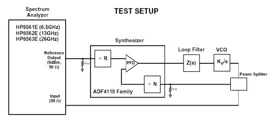
Figure 4.66: Measuring Phase Noise with a Spectrum Analyzer
