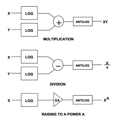
Figure 4.13: Multiplication Using Log Amps
