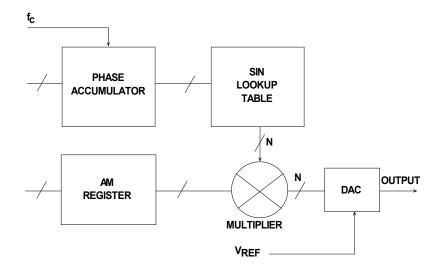
Figure 4.45: Amplitude Modulation in a DDS System
