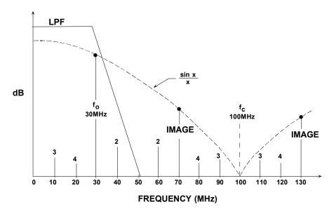
Figure 4.43: Aliasing in a DDS System
