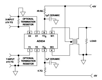
Figure 4.19: Transformer Coupled AD834 Multiplier
