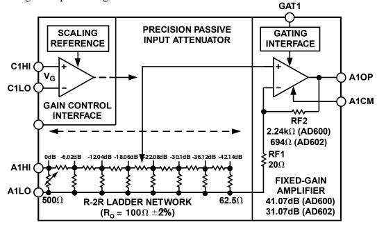
Figure 4.34: X-AMP Block Diagram
