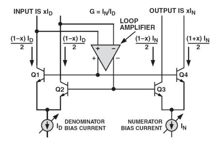
Figure 4.32: Translinear Variable Gain Cell
