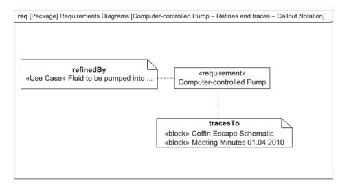
Figure 5.59 Example requirement diagram showing «refine» and «trace» relationships using callout notes
