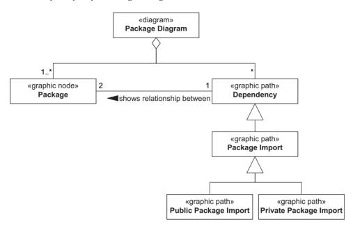
Figure 5.36 Partial meta-model for the package diagram
