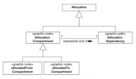
Figure 5.96 Partial meta-model for allocations
