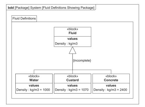
*Figure 5.41 Example block definition diagram showing a* package
