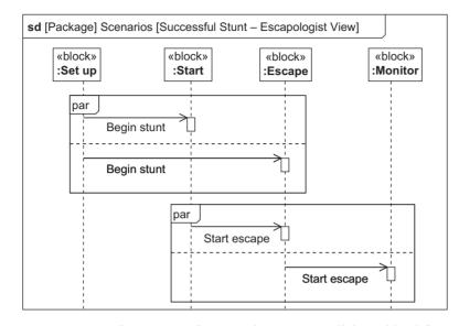
Figure 5.68 Example sequence diagram showing a parallel combined fragment
