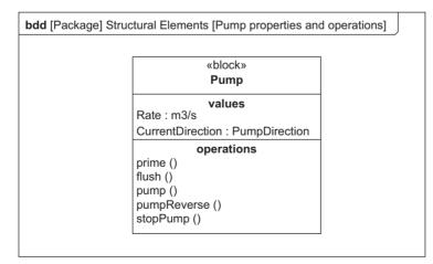
Figure 5.64 Example block definition diagram showing Pump properties and operations
