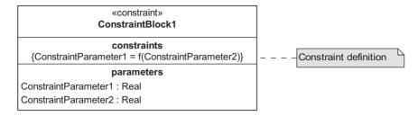
*Figure 5.43 Summary of parametric diagram notation – definition of constraint block*
