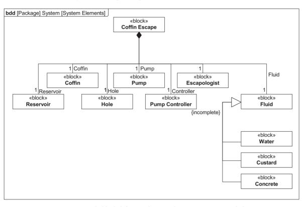
Figure 5.15 Example block definition diagram showing main structural elements of the Coffin Escape Stunt
