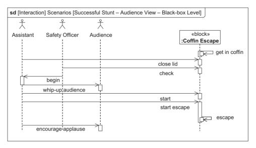
Figure 5.73 Example sequence diagram showing actors as life lines and System as a single block
