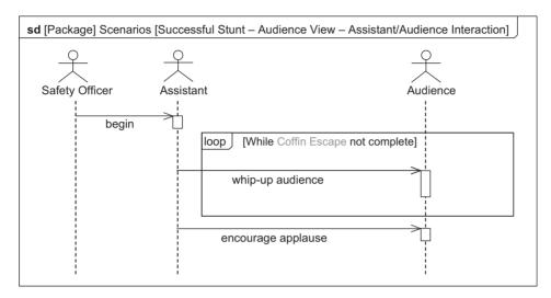
An example *sequence diagram* showing a loop combined fragment is shown in Figure 5.72.
