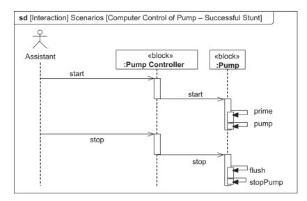
Figure 5.74 Example sequence diagram showing interactions between System Elements
