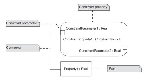
Figure 5.45 Summary of parametric diagram notation – use of constraint block
