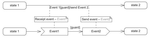
Figure 5.62 Alternative notations for receipt and send events
