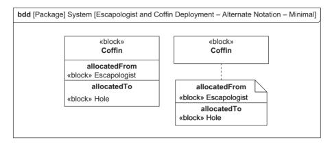
Figure 5.100 Example block definition diagram showing allocation – the minimalist approach
