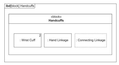
Figure 5.29 Example internal block diagrams showing owned and shared parts
