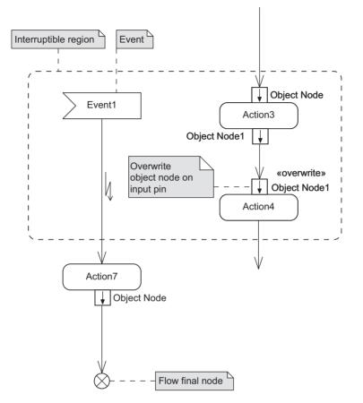
*Figure 5.81 Activity diagram notation for showing interruptible regions and use of pins rather than object nodes*
