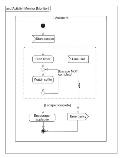
Figure 5.83 Example activity diagram showing decision, merge and interruptible region
