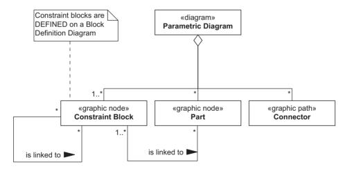
Figure 5.42 Partial meta-model for the parametric diagram
