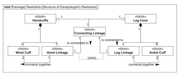
*Figure 5.28 Example block definition diagram showing modelling of owned and shared parts*
