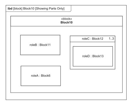
Figure 5.25 Example internal block diagram used to show its relationship to block definition diagram
