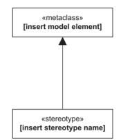
Figure 5.5 "Rubber stamp" diagram for stereotype definition
