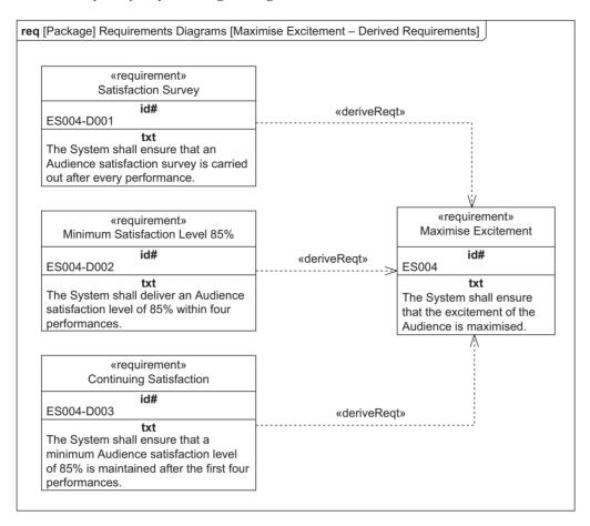
Figure 5.56 Example requirement diagram showing derived Requirements
