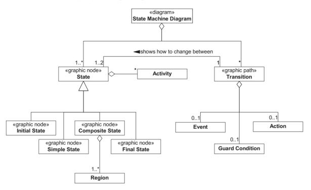
Figure 5.60 Partial meta-model for the state machine diagram
