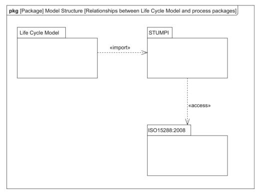
Figure 5.40 Example package diagram showing relationships between model packages
