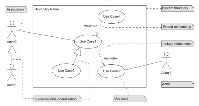
The notation that is used on *use case diagrams* is shown in Figure 5.87.
