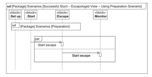
Figure 5.70 Example sequence diagram showing the use of a reference combined fragment
