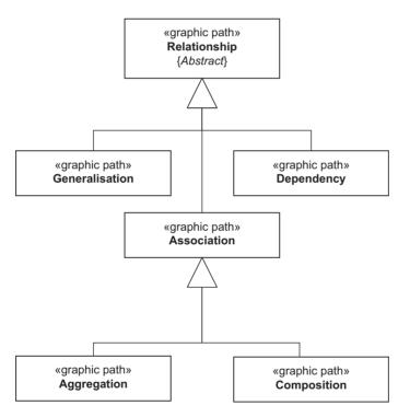
Figure 5.13 Partial meta-model for the block definition diagram showing types of relationship
