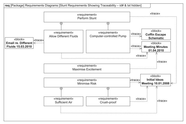
Figure 5.57 Example requirement diagram showing «trace» relationships
