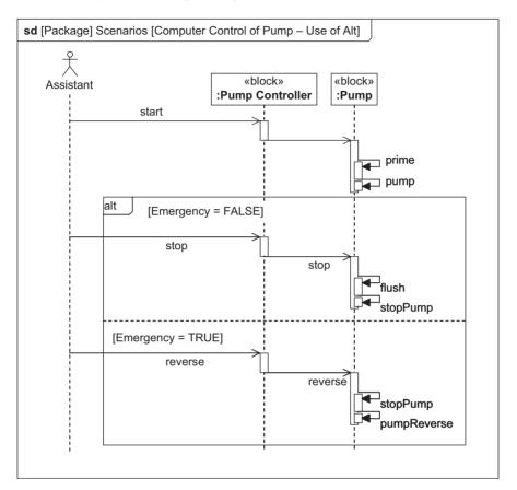
Figure 5.71 Example sequence diagram showing the use of the alternative combined fragment
