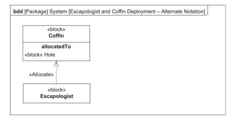
Figure 5.99 Example block definition diagram showing allocation using compartments
