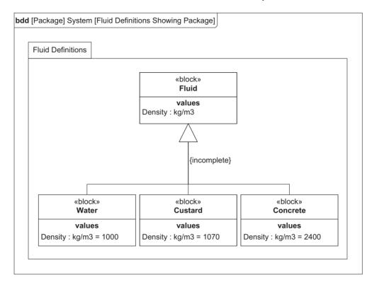
Figure 5.16 Example block definition diagram showing block properties with default values
