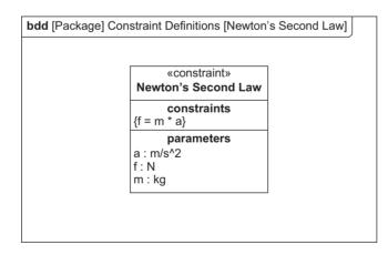
Figure 5.44 Example block definition diagram showing constraint block definition
