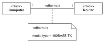
Figure 5.8 Example of stereotype usage with tags shown in comment
