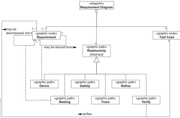
Figure 5.53 Partial meta-model for the requirement diagram
