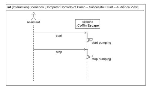
Figure 5.75 Example sequence diagram showing equivalent black box Scenario
