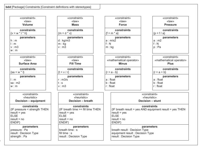
Figure 5.47 Example block definition diagram showing parametric constraints with stereotypes showing type
