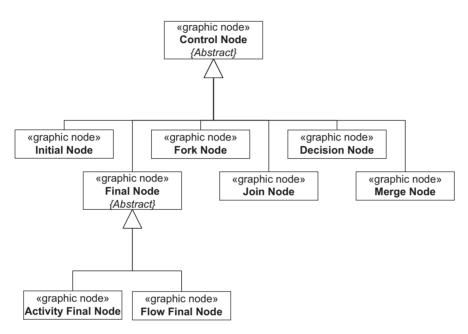
Figure 5.78 Expanded partial meta-model of the activity diagram, focusing on 'Control Node'
