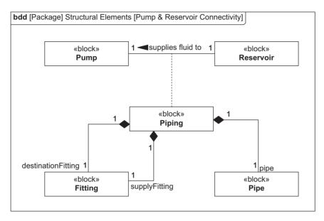
*Figure 5.33 Example block definition diagram showing connectivity using an association block*
