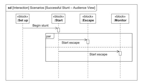
Figure 5.76 Example sequence diagram showing use of parallel combined fragment
