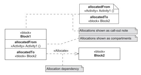
Figure 5.97 Summary of allocation notation on a block definition diagram
