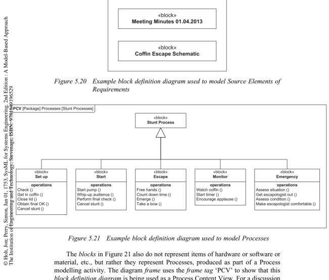
Figure 5.21 Example block definition diagram used to model Processes
