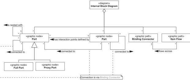
Figure 5.22 Partial meta-model for the internal block diagram
