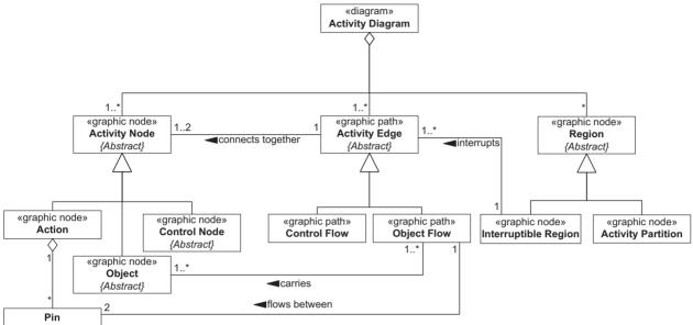
Figure 5.77 Partial meta-model for the activity diagram
