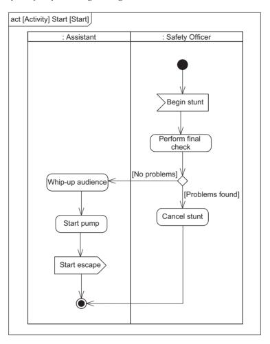
Figure 5.85 Activity diagram showing multiple activity partitions
