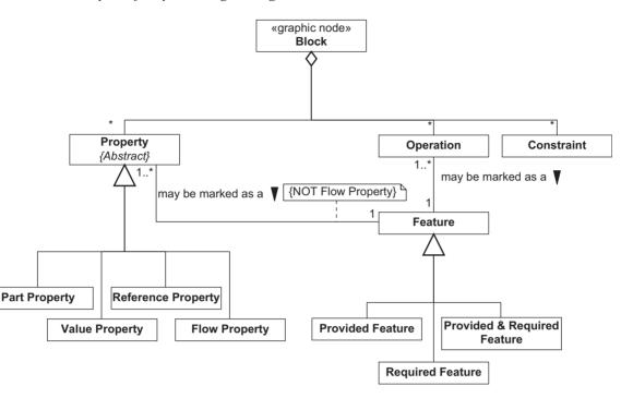
Figure 5.11 Partial meta-model for the block definition diagram showing block elements
