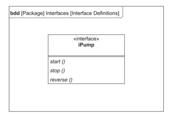
Figure 5.31 Example block definition diagram defining the iPump interface
