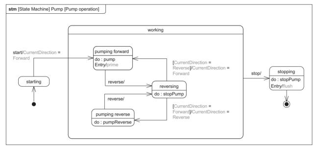
Figure 5.65 Example state machine diagram showing pump behaviour
