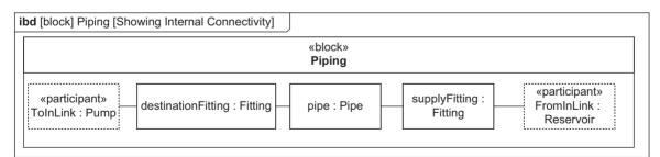
Figure 5.34 Example internal block diagram showing structure of Piping
