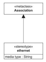
Figure 5.7 Stereotype with tag definition
