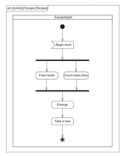
Figure 5.84 Example activity diagram showing fork nodes and join nodes
