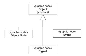
Figure 5.79 Expanded partial meta-model for the activity diagram, focusing on 'Object Node'
