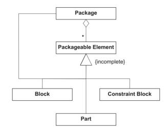
*Figure 5.39 Relationships between package diagram elements and the rest of the SysML*
