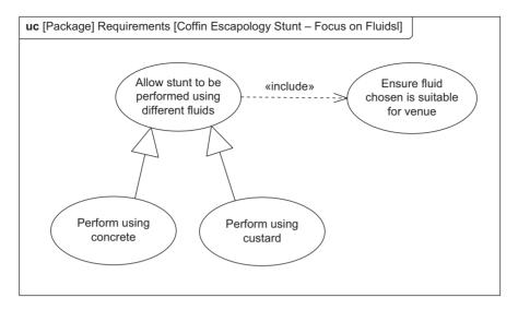
Figure 5.88 Example use case diagram showing generalisation
