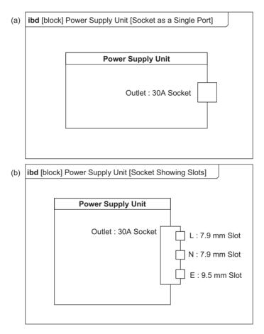
Figure 5.35 Example internal block diagram showing nested ports
