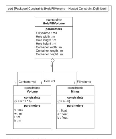
Figure 5.50 Example block definition diagram showing how higher level constraints can be constructed for the Coffin Escape Stunt
