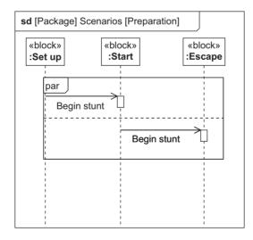
*Figure 5.69 Example sequence diagram defining common functionality to be referenced*
