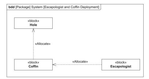
Figure 5.98 Example block definition diagram showing allocation using a dependency
