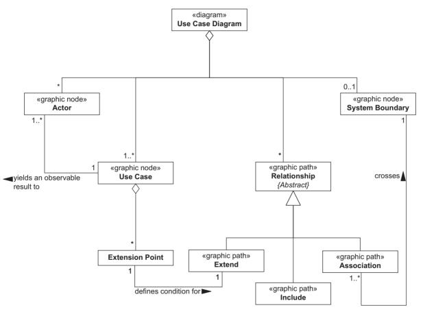
Figure 5.86 Partial meta-model for the use case diagram
