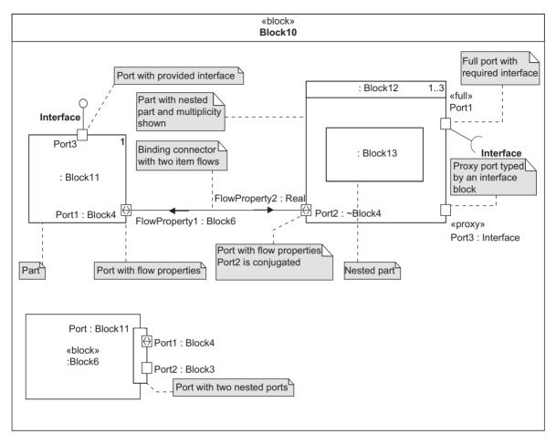
Figure 5.23 Summary of internal block diagram notation
