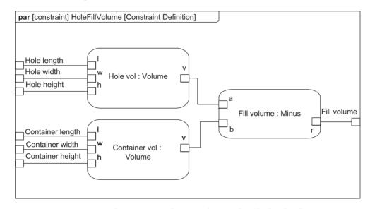
Figure 5.51 Example parametric diagram showing how higher level constraints can be constructed for the Coffin Escape Stunt
