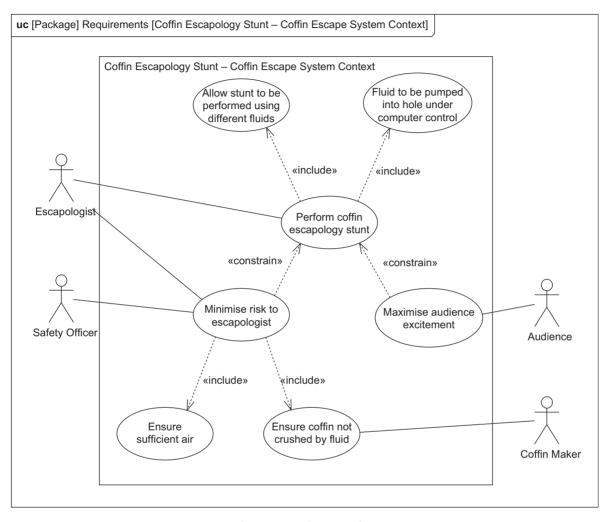
Figure 5.89 Example use case diagram showing System Context
