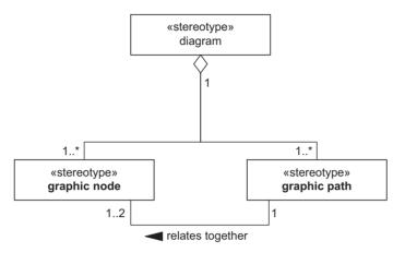
Figure 5.2 Structure of each SysML diagram
