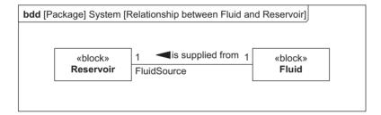
Figure 5.19 Example block definition diagram showing a reference property explicitly as an association
