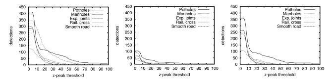
Figure 7: Pothole detections per class for varying z-peak threshold. (a) up to and including z-peak filter, (b) up to and including xy-ratio filter with  $t_x = 1.5$  (c) up to and including speed vs. z ratio filter, with  $t_x = 2.5$  and  $t_s = 5$ .
