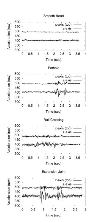
Figure 5: Sample accelerometer traces of common event types.
