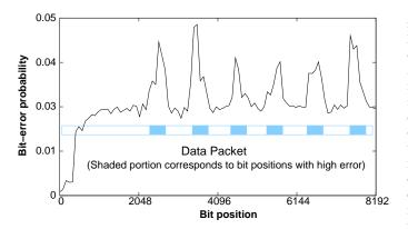
Figure 1: Distribution of bit-error probability within a packet computed over the set of packets received in error during the experiment. The error packets were modulated at 54 Mbps with a size of 1024 bytes.
