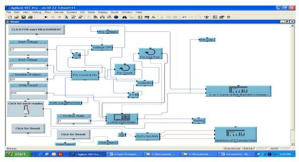
Figure 2. Main programme (Block diagram)
