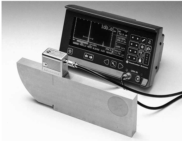
Fig. 50 Range: 250 mm with a WB 60-2 on V1 block
