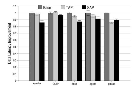
Figure 6.15: Improvement in data reference latency. From left to right, the three bars for each benchmark present the baseline system, TAP, and SAP, respectively.
