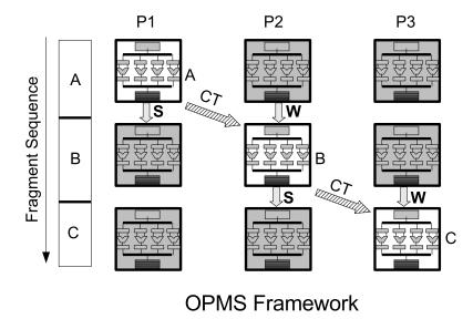
Figure 3.1: An example of OPMS execution. Inactive cores are marked by a shading.
