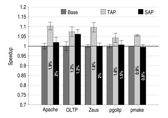
Figure 6.19: Speedup from CSP Techniques. For each benchmark, three bars show the result for the baseline (left), TAP (middle), and SAP (right), respectively. *Labels on TAP and SAP bars represent the runtime overhead of computation transfer*
