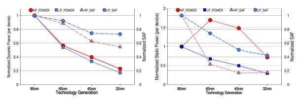
*(a)* Dynamic power trend and SAF due to dynamic *(b)* Static power consumption trend per device and SAF power exclusively. due to static power exclusively.
