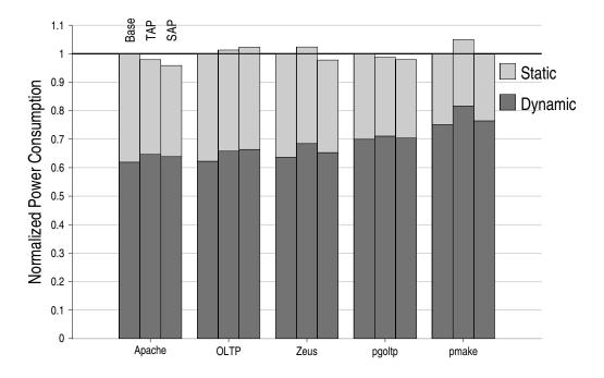
Figure 6.28: Normalized Power Consumption. Three bars for each benchmark show the results for the baseline (left), TAP (middle), and SAP (right), respectively. Each bar is also broken down to show the contribution from the dynamic power (bottom), and the static power (top).
