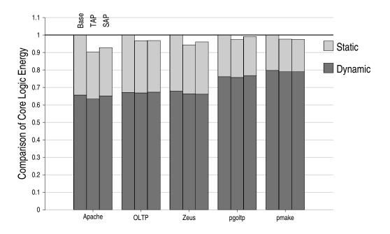
Figure 6.23: Comparison of Energy Expenditure in the Core Logic. For each benchmark, three bars show the result for the baseline system, TAP and SAP, respectively. Each bar is broken down to show the dynamic (bottom) and static energy (top) components
