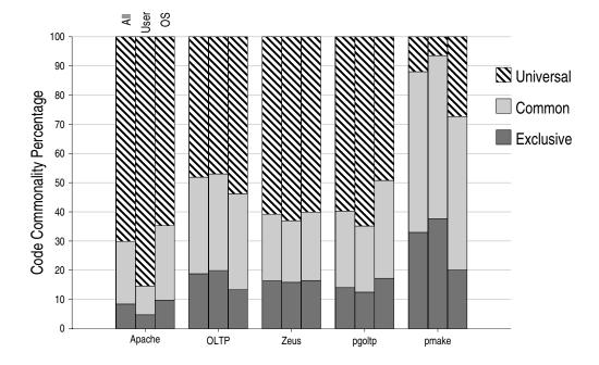
Figure 4.1: Code Commonality Characteristics for a multicore with 8 cores. *Each 64-byte static instruction block is marked* Universal *if accessed by all the cores,* Common *if accessed by more than one core, and* Exclusive *if accessed by only one. The left bar shows the commonality profile for the entire execution, the middle bar shows commonality for only user code, and the right bar shows the commonality for OS code.*
