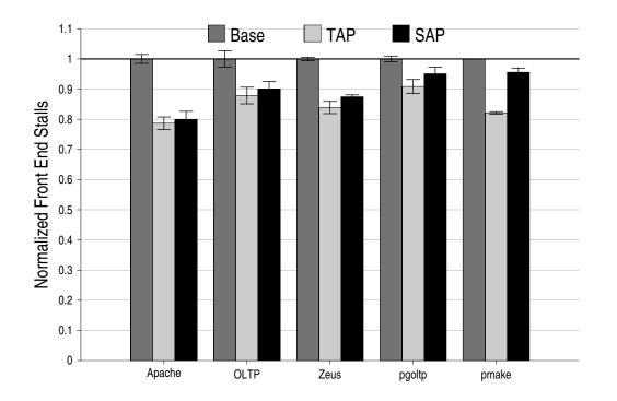
Figure 6.7: Front end stall events comparison. The three bars for each benchmark represent results for the baseline system, TAP and SAP, respectively (left to right).
