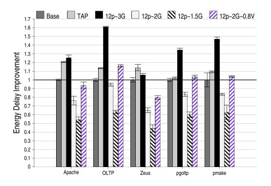
Figure 6.33: Energy delay comparison 12-core multicore configurations. From left to right, six bars in each benchmark shows the results for the baseline 8 core system, TAP, and several 12 core systems operating at different frequency levels indicated in their respective labels. The rightmost bar shows the result for a voltage scaled (0.8V) 12 core system.
