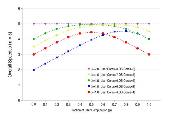
Figure 2.6: Speedups in server applications with varying user computations. The fraction of time spent in the user computation ( $\beta$ ) is varied from 0 to 1.0. The speedups are shown for  $\eta = 5$ .
