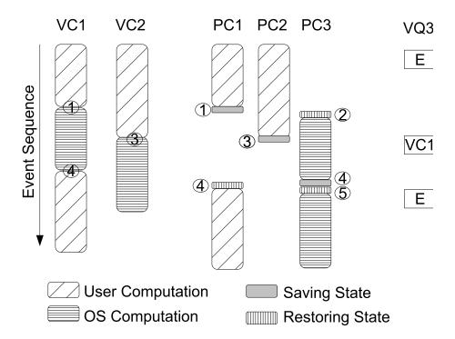
Figure 4.4: CSP Implementation: Handling Contention. Two virtual cores, VC1 and VC2, are assigned to an OPMS with three physical cores: PC1, PC2, and PC3. The user computation from VC1 and VC2 are assigned to PC1 and PC2, respectively, while the OS computation from both the virtual cores are assigned to PC3.
