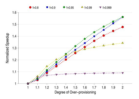
Figure 2.4: Impact of over-provisioning in asymmetric multicore speedup. Degree of overprovisioning indicates the ratio of available compute resources to the allowable active resources. The speedups are normalized to the speedup obtained when the degree of over-provisioning equals one.
