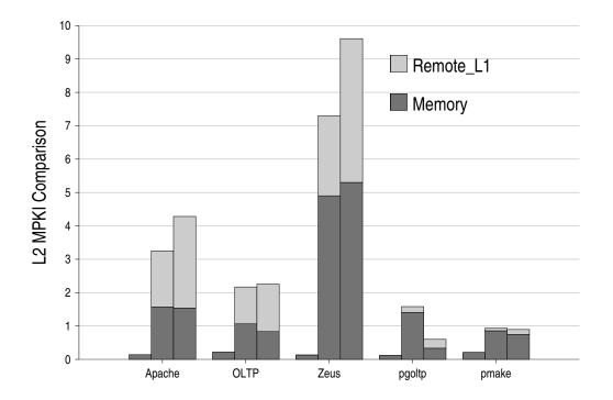
Figure 6.4: L2 misses presented as misses per kilo instructions (MPKI). From left to right, the three bars represent instruction fetch misses, data cache misses from load operations, and data cache misses from store operations, respectively. Each bar is also broken into two parts showing the misses that source data from the main memory and remote L1, respectively.
