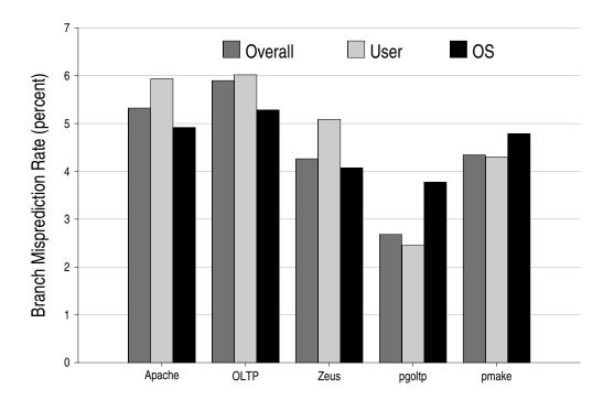
Figure 6.16: Branch Mis-prediction Rates (percent) in the baseline system. From left to right, three bars for each benchmark shows the result for the overall miss rate, miss rates in user code, and the miss rate in OS code, respectively.
