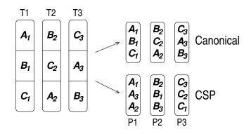
Figure 4.2: Computation Spreading vs. the Canonical Model for mapping computation fragments from a thread.  $A_1$ ,  $A_2$  and  $A_3$  denote similar fragments from different threads;  $A_1$ ,  $B_1$  and  $C_1$  denote dissimilar fragments of the same thread.
