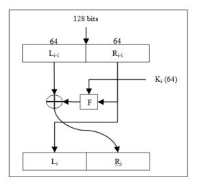
Figure 5. One Round Encryption Structure
