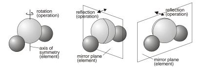
Each symmetry operation has a corresponding *symmetry element*, which is the axis, plane, line or point with respect to which the symmetry operation is carried out. The symmetry element consists of all the points that stay in the same place when the symmetry operation is performed. In a rotation, the line of points that stay in the same place constitute a *symmetry axis*; in a reflection the points that remain unchanged make up a *plane of symmetry*.
