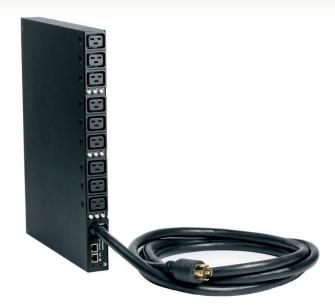
Figure 3. The 1U Switched and Monitored PDU features nine C19 receptacles on the front and three C13 receptacles on the back.
